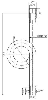
Designed to protect the gauge from media at high temperatures, like steam. Also to reduce the effect of sudden changes in pressure. For initial installation must fill the siphon with water or other equivalent liquid
